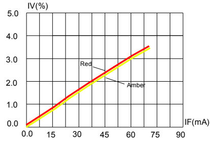
FIG.2 RELATIVE LUMINOUS INTENSITY VS. FORWARD CURRENT
