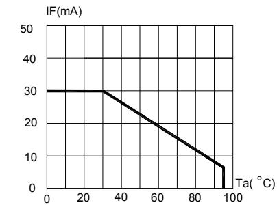
FIG.5 MAXIMUM FORWARD DC CURRENT
