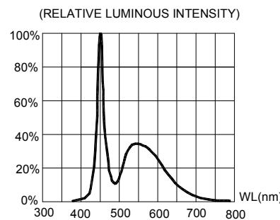
FIG.4 RELATIVE LUMINOUS INTENSITY VS.
